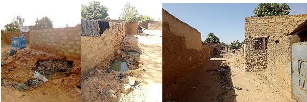
Figure 17. Streets in the non-loti areas of Somgandé with cesspits full of wastewater and garbage (left) and visible stormwater runoff (right)
