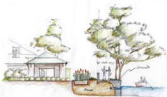
New walkway along the canals in combination with sandbody to clean the run-off water
