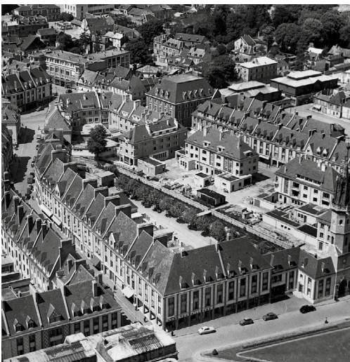
6. Evreux (27). Aerial view of the reconstruction in the 1950s. Urban planning comprised of townhouses aligned with the street, including widened streets and plots. Return to the old block-style plan.
