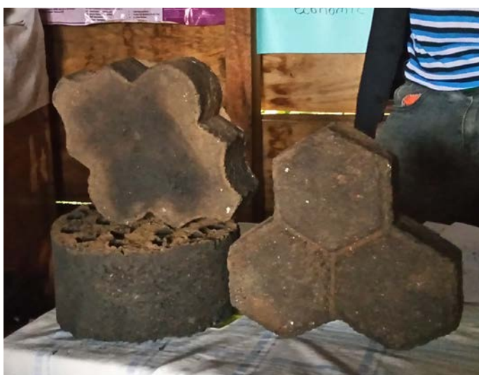
Paving stones made of plastic (and a briquette) in Kasanvu
