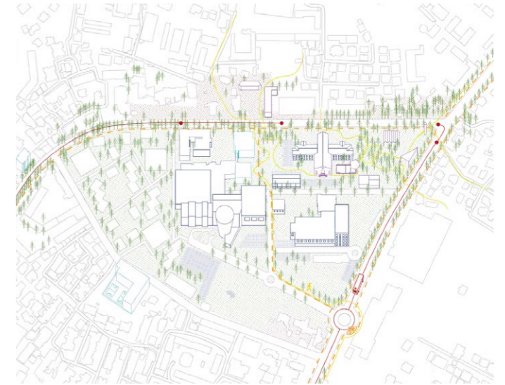
Proposed accessibility to the area and within the district: in red, autobus lines, and in yellow, pedestrian paths (Ministry of Culture)
