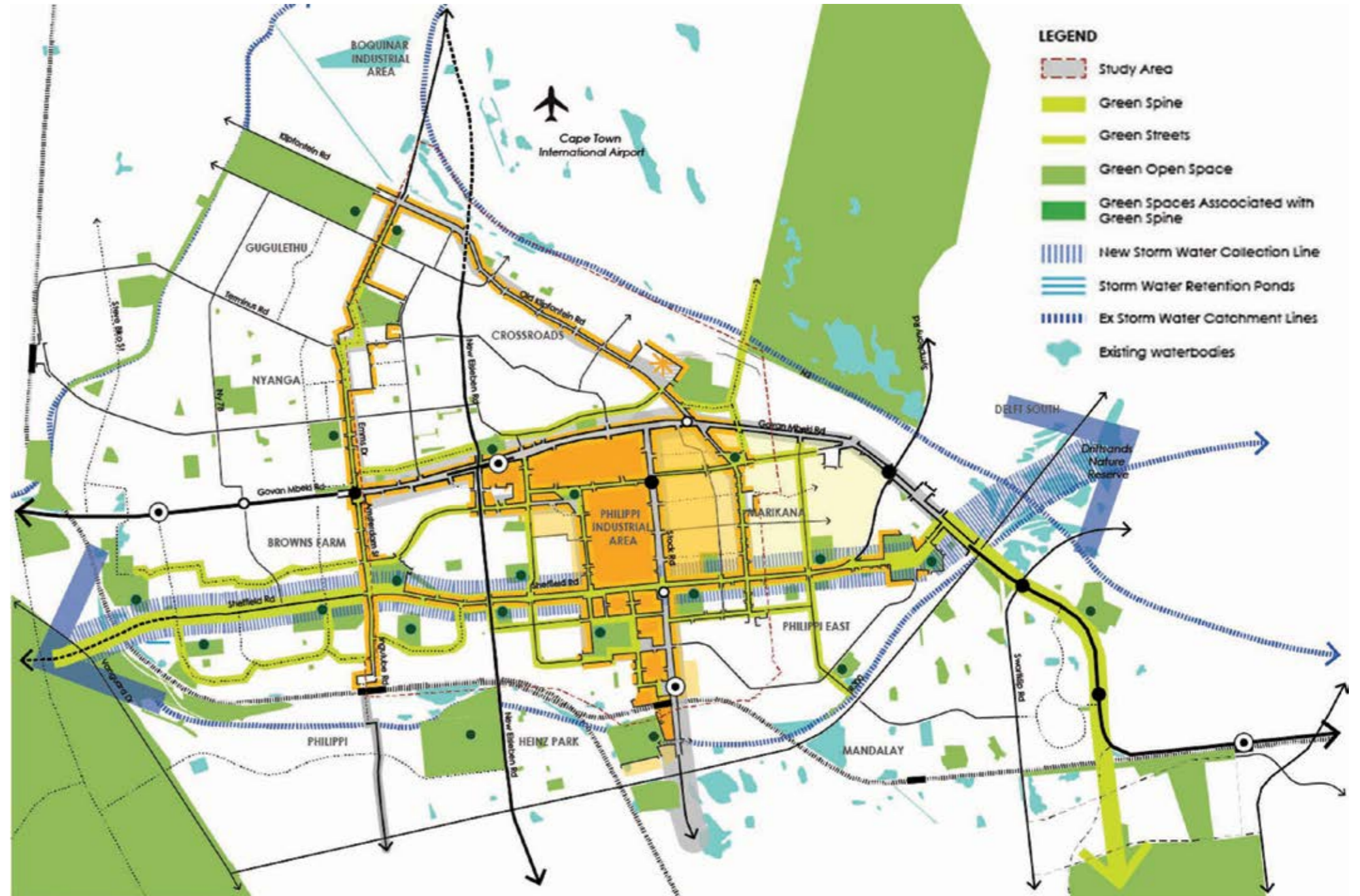
Figure 35. A series of retention ponds are situated along Sheffield Road. Despite this the whole area is prone to flooding. There is a fragmented open space network throughout the POA and its surrounds, highlighted in green (source: supplied by the CoCT).
