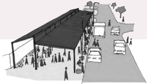
Figure 62. The Sustainable Livelihoods Foundation's (SLF) proposal for informal trading areas with access to shelter, storage, visibility and utilities such as water and electricity (source: SLF, 2018).
